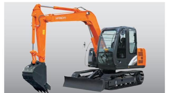
Note: The pictured ZX70 is equipped with an optional blade.
