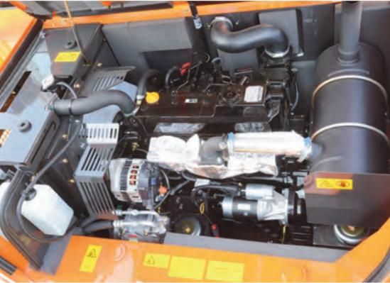
New electronically-controlled engine
