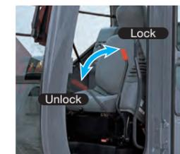
Pilot control shut-off lever
