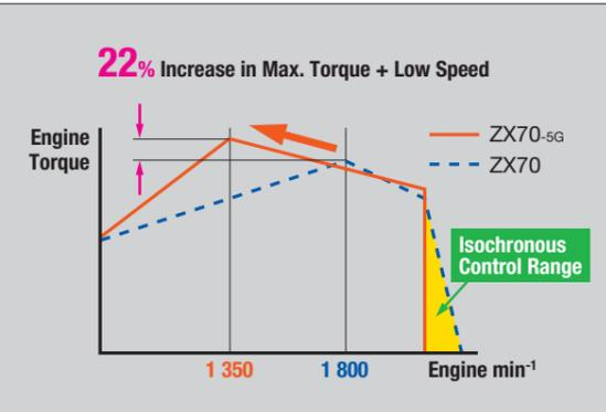
Engine torque vs. engine min<sup>-1</sup>
